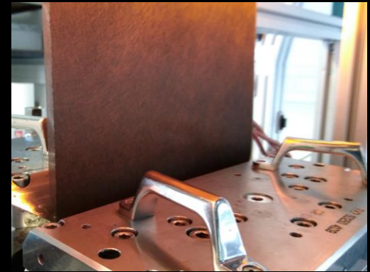
GDL Impregnation with FMP Slot Die
